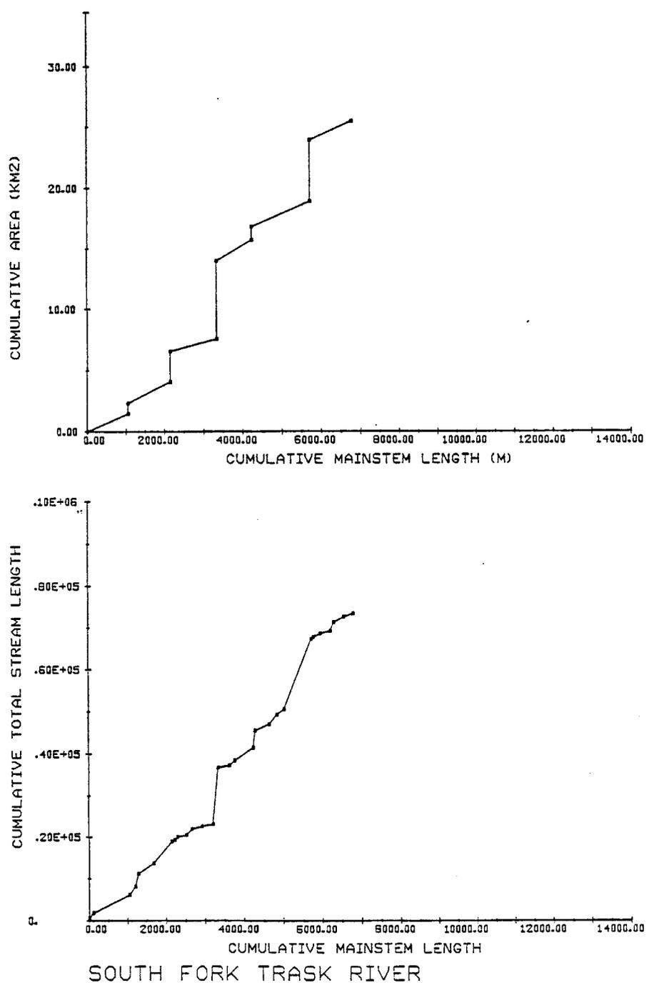
Figure 16. Representative plot (South Fork Trask) of cumulative total stream length vs. cumulative mainstem length and cumulative area vs. cumulative mainstem length proceeding from upstream to downstream on the mainstem.
