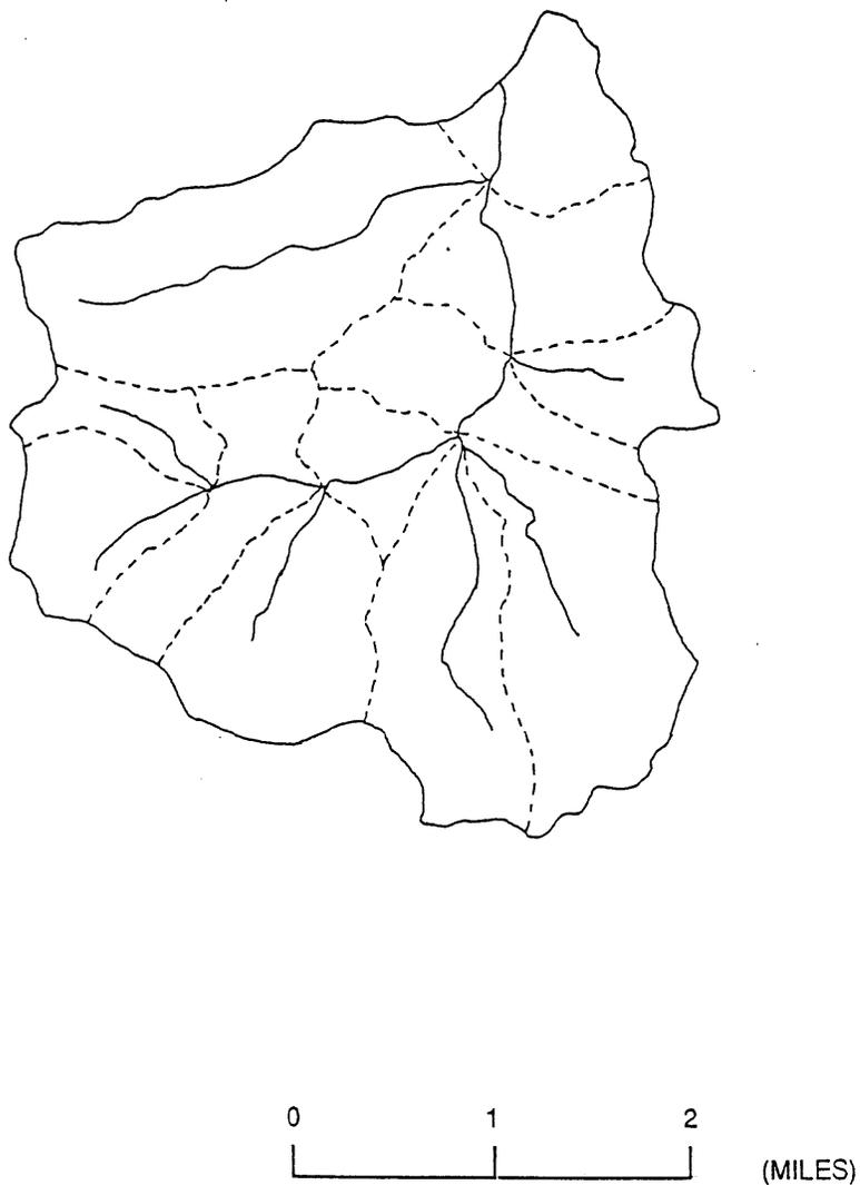
Figure 5. The blue-line drainage network (solid line) and sub-basin boundaries (dotted-line) for the South Fork Trask River. Points at which to initiate integration of daily solar radiation load are spaced at 880 ft intervals along entire blue-line network.
