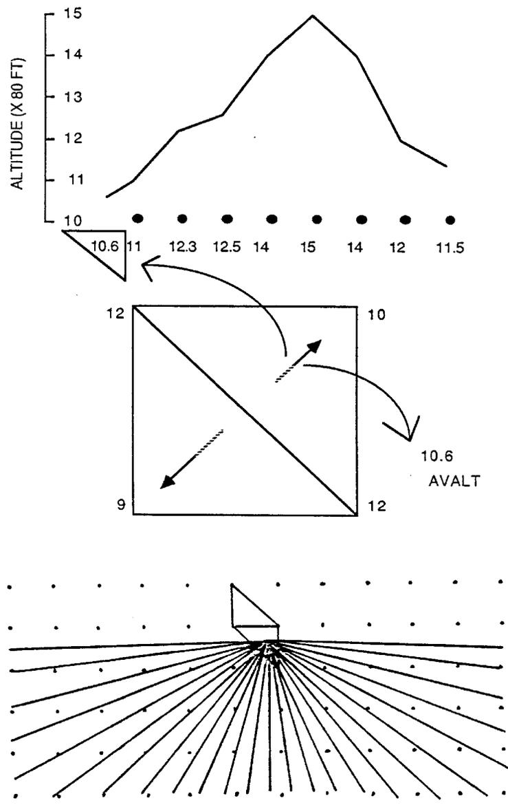
Figure 4. Computer search through the altitude grid for topographic ridges providing maximum shading factor at increments (7.5 degrees) of solar movement along meridian. A search on the equinox is diagrammed.
