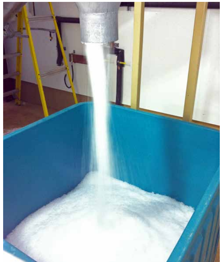
The flake ice machine at the White Salmon Fish Processing Center is capable of producing 10 tons of ice per day. Above is a tote being filled from the ice machine.
