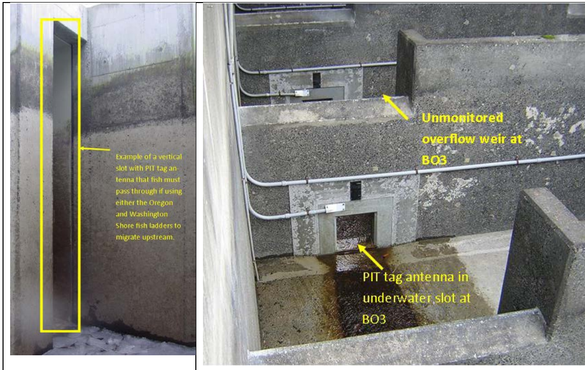
Figure 2. Pictures of the two types of PIT tag antennas at Bonneville Dam. The vertical slot antennas are at the upper end of both ladders, while the underwater antennas are in the lower parts of the ladders. Photos courtesy of Alan Brower of PTAGIS.
